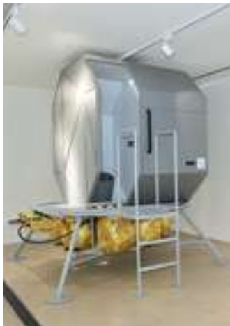
pee power live test - Bio Brennstoffzellen erzeugen aus Urin Strom. Bristol Robotics Laboratory design by EOOS
