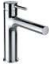
Single lever basin mixer, projection 140 mm, fixed spout, with pop-up waste / without pop-up waste
