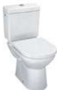
Floorstanding WC, close-coupled, washdown, with flushing rim, outlet horizontal 670 x 360 x 420 (400) mm
